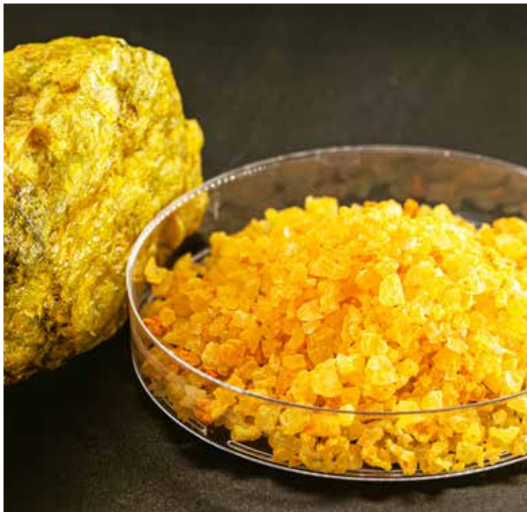
Uranium ore (left) and uranium ore concentrate in the form of uranyl nitrate (right)
