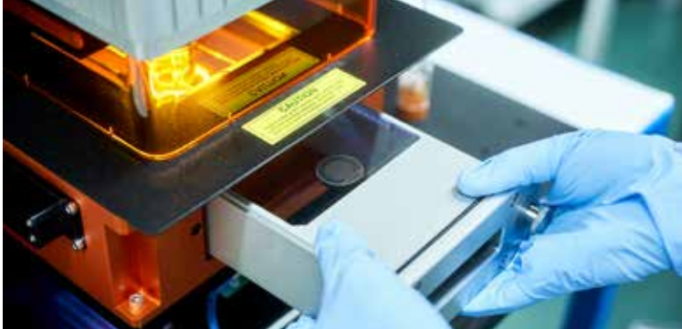
A nuclear forensics sample ready for laser ablation analysis ©European Commission
