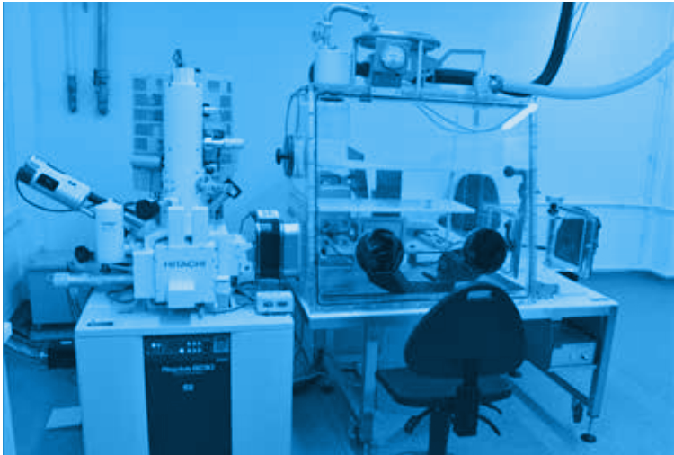
Figure 5-7. NFL-R0 scanning electron microscope connected to a glovebox provided by IFIN-HH.
