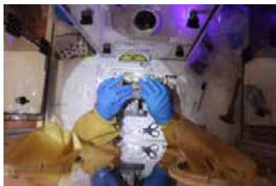
Figure 4-3. Nuclear scientist performing forensics analysis on contaminated evidence within a glovebox (photo provided by IFIN-HH, Romania).
